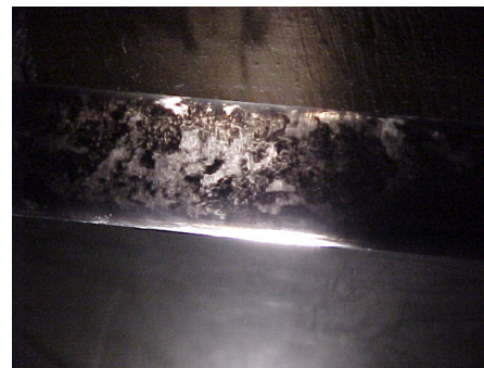
Breakdown of biofilm begins with mixed oxidants
